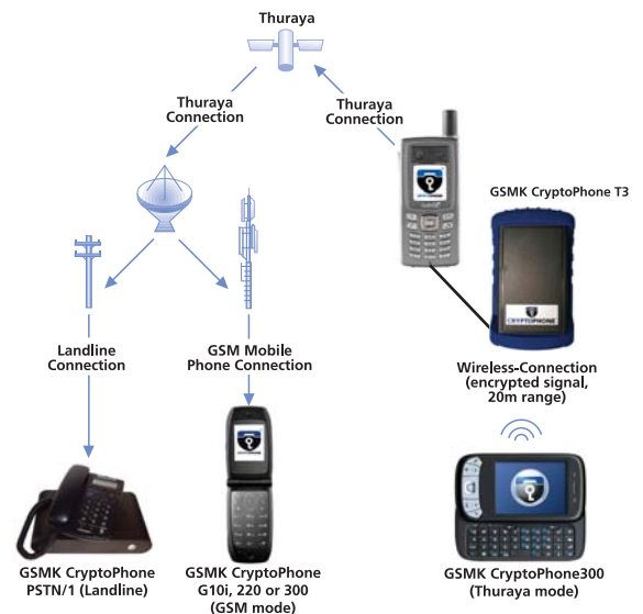
FIGURE (2): T3 WIRELESS CONNECTION USING SO-2510, T3, AND CP300
