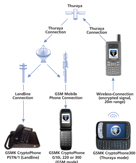
FIGURE (3): WIRELESS CONNECTION USING ONLY SG-2520 AND CP300
